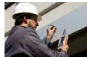
Measurement of anodizing coating on aluminum on a facade
