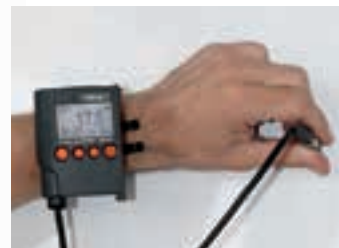
Wristband for MPOR-FP instruments for one-hand operation
