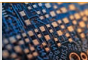
Printed circuit boards: Au/Ni/Cu/PCB
