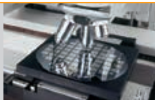
Wafer: Hardness determination on the gold coating
