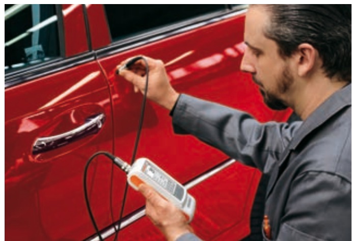
Measurement of car body paint thickness using the dual probe FD10.
