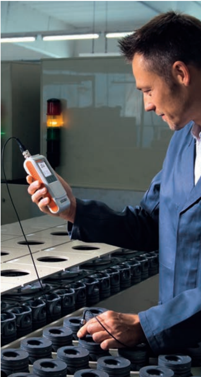
Quality monitoring on engine pistons after the manufacturing process using the FTA3.3H probe.
