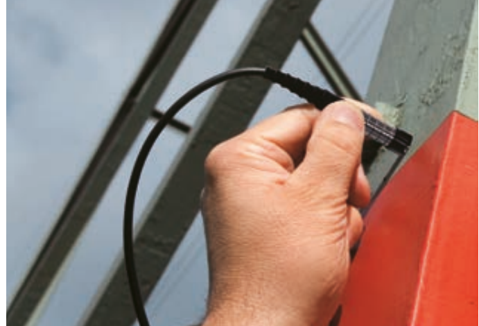
Duplex measurement of paint-zinc coatings with the probe FDX13H.
