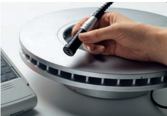
Measurement of zinc powder coating with the two-pole probe V7FKB4.
