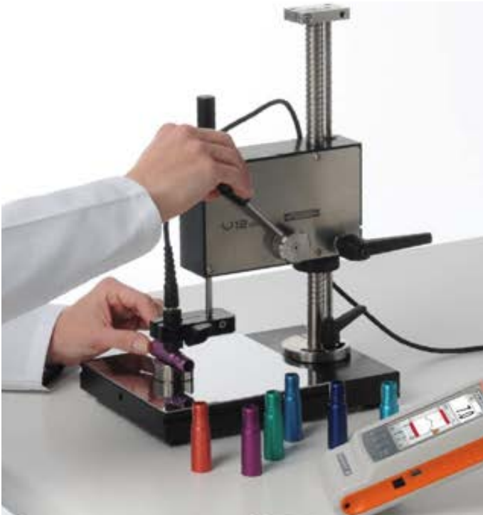
Measurements of anodized coatings on sleeves using the curvature-compensated probe FTD3.3, clamped into the support stand V12 Base.
